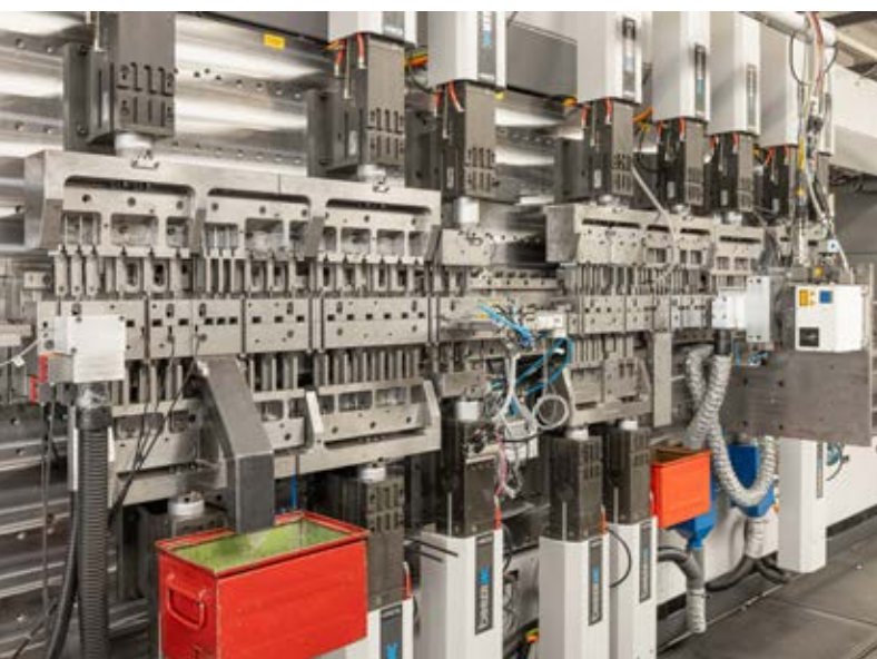
Production of the connector involves approximately 100 different manufacturing steps on the Bihler BIMERIC BM 4500.
