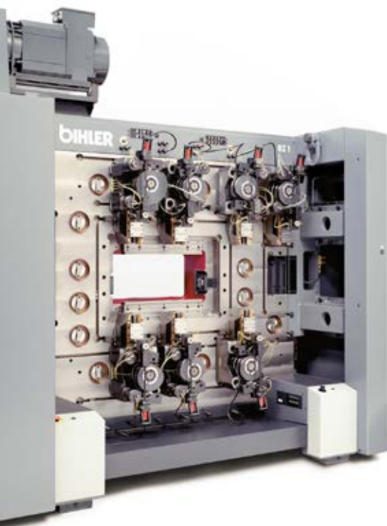
The first BZ linear forming/processing center provides the basis for the efficient manufacture of assemblies.
