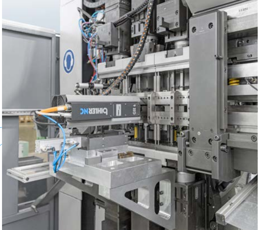
The linear tool for the new Bihler GRM-NC was developed in-house by Industrias Huerta.
