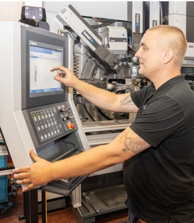
Peter Josefsson, Head of Maintenance at EWES, at the controller for the new Bihler GRM-NC.
