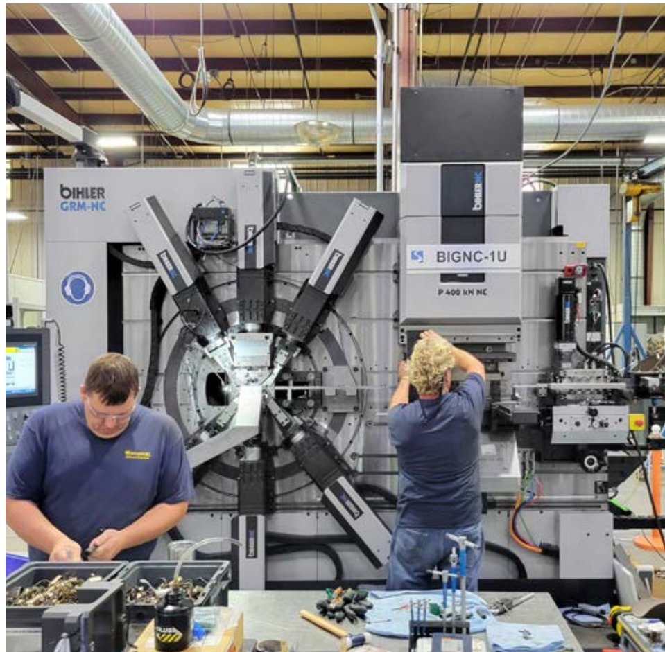
Focusing on the customer's needs: Thanks to the short setup times, it is even possible to manufacture smaller batch sizes efficiently on the Bihler GRM-NC.
