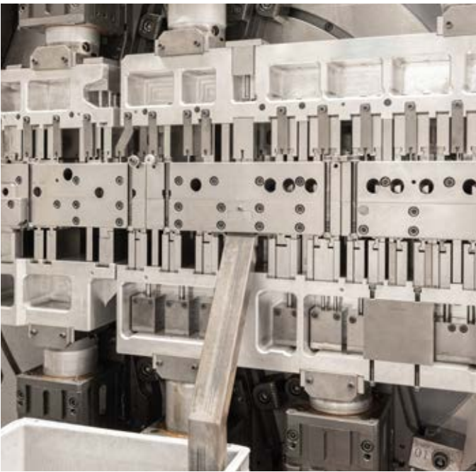
Connectors for charging electric vehicles are manufactured on a new Bihler GRM-NC. The linear tool used for this was designed in-house by M.S.Ambrogio itself.
