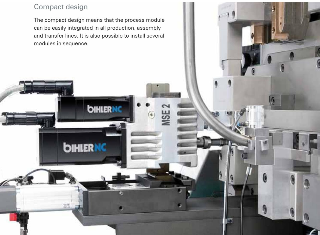
MSE 2 with integrated lifting device as a sub-system (output 120/min).
