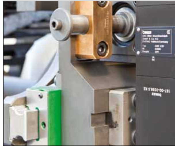
Freely programmable processing positions of the GSK KS units
