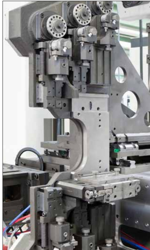
Welding process module without contact welding unit and kits for strip guidance
