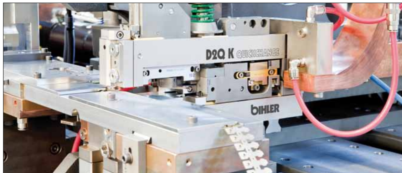
Welding process module with integrated welding tool and guide set
