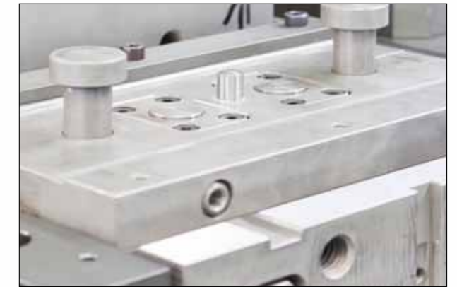
Rapid locking system for all replaceable components
