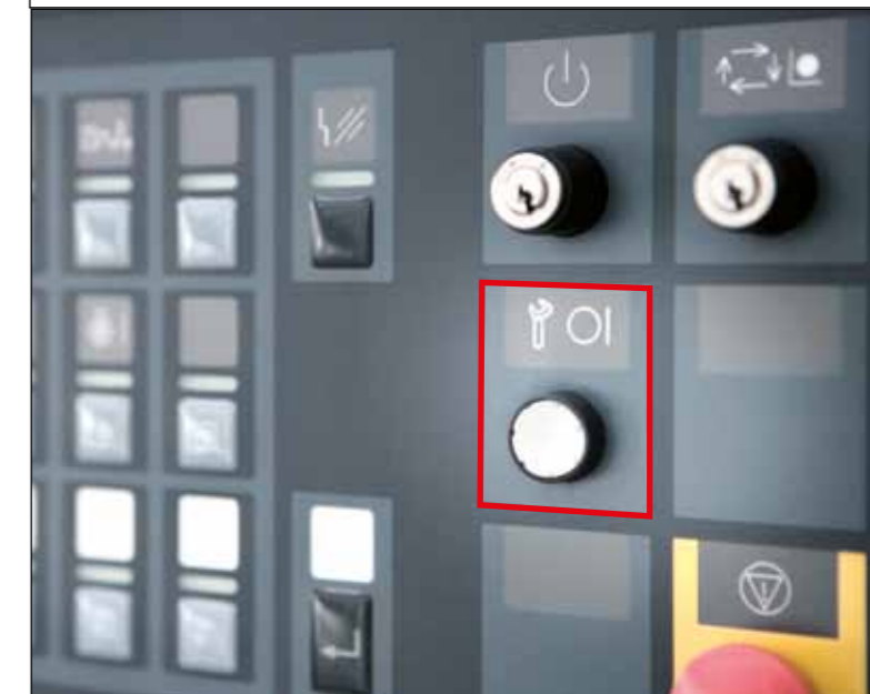
When prompted, activate the secure link by pressing this button on the operating console on the control unit.
